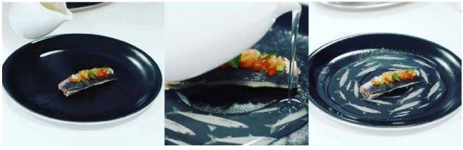
Figure 2. Plate that changes appearance thanks to the use of black thermochromic pigments. Initially, the plate is black (left); when a warm liquid is poured (center), the black thermochromic pigments become transparent; in the end, the plate's appearance is different (right). The prototype in the image was developed by EureCat (www.eurecat.org).
